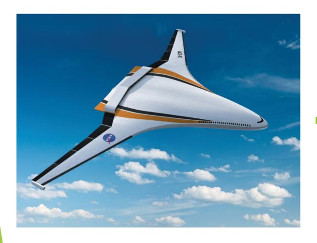
This idea for a possible future aircraft is called a "hybrid wing body" or sometimes a blended wing body. In this design, the wing blends seamlessly into the body of the aircraft, which makes it extremely aerodynamic and holds great promise for dramatic reductions in fuel consumption, noise and emissions.
