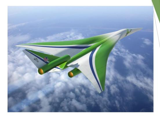
Our ability to fly at supersonic speeds over land in civil aircraft depends on our ability to reduce the level of sonic booms. NASA has been exploring a variety of options for quieting the boom, starting with design concepts and moving through wind tunnel tests to flight tests of new technologies. This rendering of a possible future civil supersonic transport shows a vehicle that is shaped to reduce the sonic shockwave signature and also to reduce drag.
