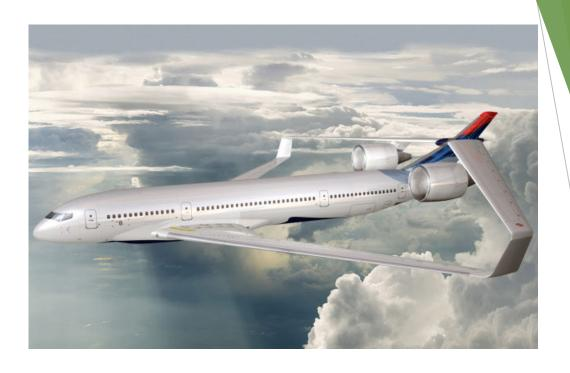
► Lockheed Martin's advanced vehicle concept proposes a box wing design, which is now feasible thanks to modern lightweight composite (nonmetallic) materials, landing gear technologies and other advancements. Its Rolls Royce Liberty Works Ultra Fan Engine achieves a bypass ratio (flow of air around engine compared to through the engine) nearly five times greater than current engines, pushing the limits of turbofan technology to maximize efficiency.
