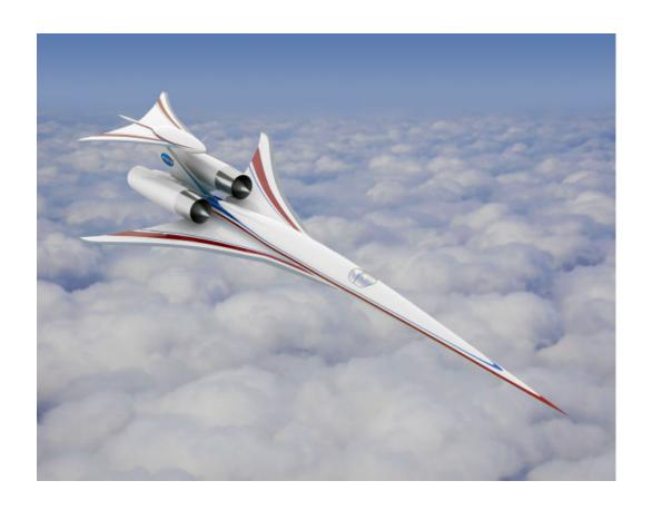
This concept of an aircraft that could fly at supersonic speeds over land is being used by researchers, especially at NASA's Langley Research Center, to continue to test ideas on ways to reduce the level of sonic booms. Its technologies - the F-100-like propulsion system, a tail blister, and the overall shape - are combined to achieve a lower target perceived decibel level.
